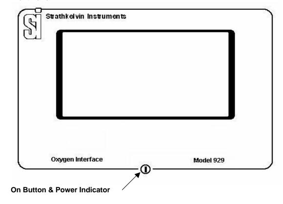
The Power button switches the interface on and off. It is disabled while measurements are being made.
